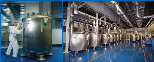
Fig. 1: Cryostorage vessels. A: Cryostorage tank, technologically modified with hover cushion brackets; B: Cryostorage facility in Sulzbach.
