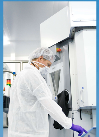
Fig. 4: Semiautomatic cryostorage system with the Fraunhofer-Cryostorage-Technology (Fa. Askion)
